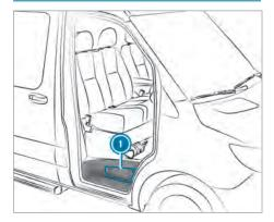
The hydraulic jack is located in side compartment
