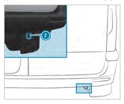
Rear towing eye (vehicles with passenger vehicle approval)
