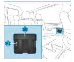
Place the mobile phone in stowage compartment (a) and connect it to USB port (a) to charge.
