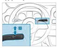
Depress the brake pedal and push the DIRECT SELECT lever upwards past the first point of resistance.
