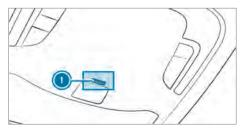
When the ATA system is armed, indicator lamp 1 flashes in the overhead control panel.
