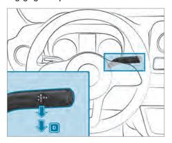
Depress the brake pedal and push the DIRECT SELECT lever downwards past the first point of resistance. Transmission position display **D** is shown in the multifunction display.
