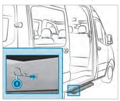
On both sides, insert spring cotters through the housing's holes and into the step as far as they will go.
