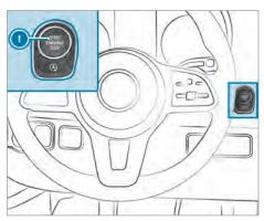
To switch on the power supply: press button nonce.
