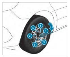
Tighten the wheel bolts or nuts evenly in the sequence indicated (1) to 6).
