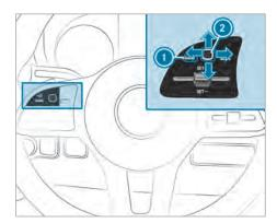
The on-board computer is operated via left-hand Touch Control 2 and back button on the left 1.
