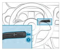
Press button 1. Transmission position display P is shown in the multifunction display.
