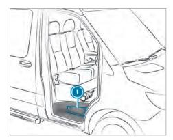
The tire-change tool kit is located in stowage compartment 1 above the step of the co-driver's door and in the stowage compartment in the footwell on the co-driver side.
