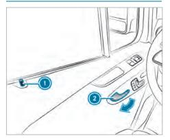
To unlock and open the front door: pull door handle ②.
