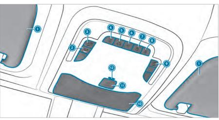
Overhead control panel for vehicles with bus equipment Sun visors lighting on/off ② ✓ Breakdown assistance call button reading light on/off Activates/deactivates 89 the bus function passenger compartment on/off reading light on/off (ii) Glasses compartment (5) Switches automatic light control on/off Switches the front interior lighting on/off
