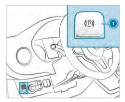
To prevent the electric parking brake from applying automatically, pull switch 1.
