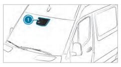
Traffic Sign Assist detects traffic signs with multifunction camera (1). It assists you by displaying detected speed limits and overtaking restrictions in the instrument cluster.
