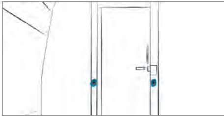
Photoelectric sensor on the sliding partition door
