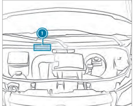
Engraved VIN ① is located underneath the hood.
