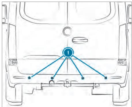
Certain driving and driving safety systems use sensors ❶ to monitor the area in front of, behind or next to the vehicle (depending on the vehicle's equipment).
