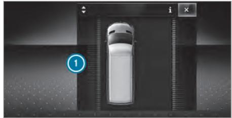
If a lane-correcting brake application from Active Lane Keeping Assist occurs, display ① appears in the multifunction display.
