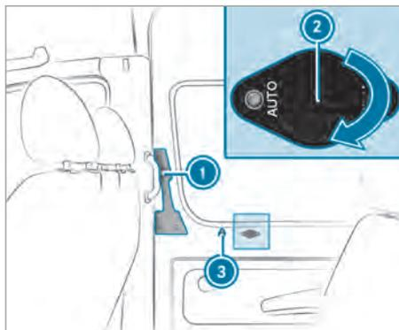
If there has been a malfunction or if the battery has been disconnected, you can use release catch **2** to disconnect the sliding door from the electric motor. Then, you can open or close the door manually.
