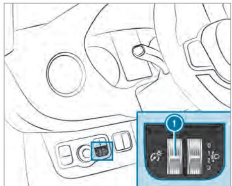
▶ Turn brightness control knob ① upwards or downwards.
