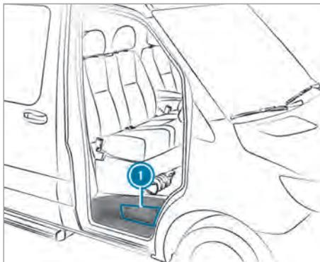
The tire-change tool kit is located in stowage compartment ① above the step of the co-driver's door and in the stowage compartment in the footwell on the co-driver side.
