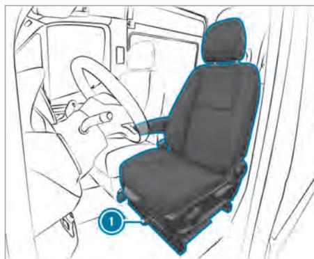
You can rotate the driver's and front passenger seat 50° and 180°. The seats engage both in and opposite to the direction of travel as well as at 50° to the exit.
