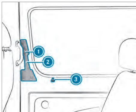
**i** Your vehicle may be equipped with a long sliding door with an intermediate detent. You can also lock the sliding door in place around halfway when opening and closing. If you do this, the door does not have to be opened fully when getting into or out of the vehicle. The sliding door is not fully engaged when in the intermediate detent.
