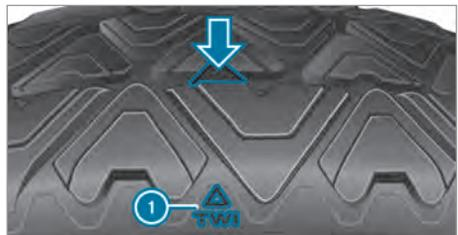
Markings ① show in which places the bar indicators (arrow) are integrated into the tire tread. They are visible as soon as the tread depth is approximately  $\frac{1}{16}$  in (1.6 mm).
