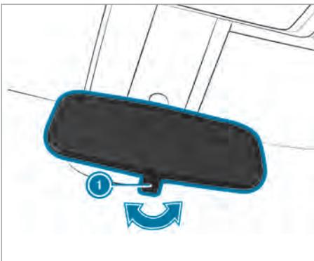
▶ **To dim the inside rearview mirror:** move anti-glare lever ① in the direction of the arrow.
