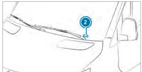
The VIN is also attached as a label on the lower section of windshield ②.
