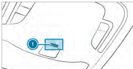
When the ATA system is armed, indicator lamp ① flashes in the overhead control panel.
