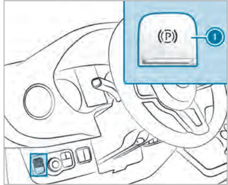
To prevent the electric parking brake from applying automatically, pull switch
