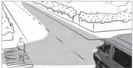
The cornering light improves the illumination of the roadway over a wide angle in the turning direction, e.g. enabling better visibility in tight bends.
