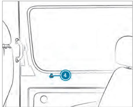
When the sliding door is locked, it can only be opened from the inside by manually unlocking locking pin ④.
