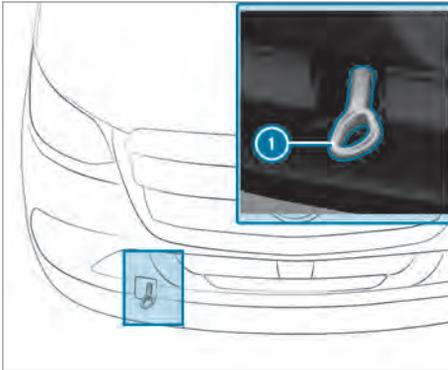
Installing and removing the front towing eye
