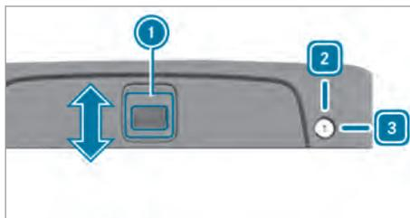
▶ **To unlock:** turn the emergency key clockwise to position ③.
