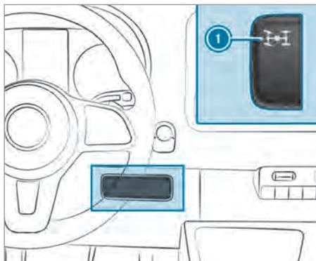
▶ **To engage/disengage:** press the upper section of switch ①.
