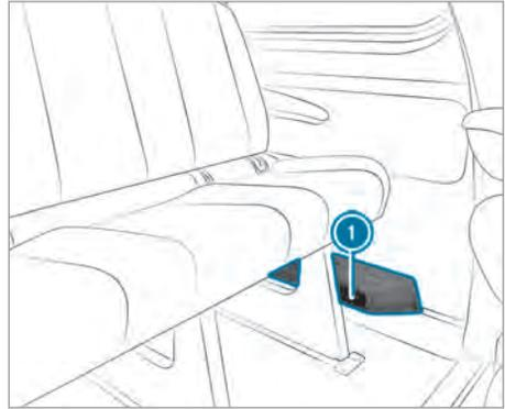
Depending on the vehicle equipment, there will be an air duct or a heater with additional air vents in the rear compartment footwell on the left-hand side ❶. No objects may be placed there. Occupants must maintain a sufficient distance due to the warm air flow and air intake.
