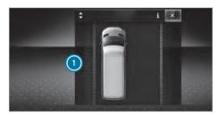
If a lane-correcting brake application from Active Lane Keeping Assist occurs, display
