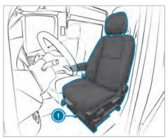
You can rotate the driver's and front passenger seat  $50^{\circ}$  and  $180^{\circ}$ . The seats engage both in and opposite to the direction of travel as well as at  $50^{\circ}$  to the exit.
