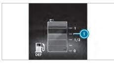
Instrument Display with color display DEF level
