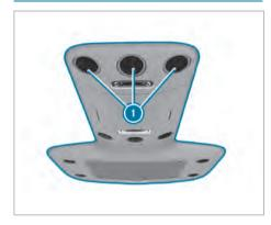
In vehicles with a rear compartment air conditioning system, adjustable air vents have been integrated in the roof air duct.
