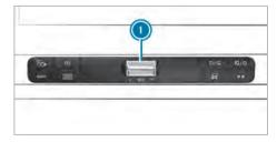
To raise/reduce the volume in steps: briefly press rocker switch ① up or down. To raise/reduce the volume continuously: press rocker switch () up or down until the desired volume is set.
