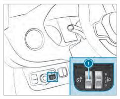
Turn brightness control knob (1) upwards or downwards.
