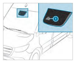
Lane Keeping Assist monitors the area in front of your vehicle with multifunction camera (). It serves to protect you against unintentionally leaving your lane. You may also be warned by a vibrating message from the steering wheel and by the status symbol flashing in the Instrument Display.
