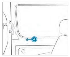
When the sliding door is locked, it can only be opened from the inside by manually unlocking locking pin ().
