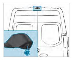
If you have activated the function in the multimedia system, the image from rear view camera appears in the multimedia system when reverse gear is selected. Dynamic guide lines show the path the vehicle will take with the steering wheel in its current position. This helps you to orient yourself and to avoid obstacles when backing up. The image from rear view camera () appears in the multimedia system when the following conditions are fulfilled:
