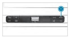
► To switch off: briefly press button ①. The k symbol appears in the status line of the multimedia system display.
