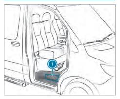
The hydraulic jack is located in side compartment ① above the co-driver door step.
