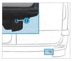
Rear towing eye (vehicles with passenger vehicle approval)
