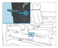
Top Tether anchorages ① are located on the back of the rear bench seat on the bench seat legs.
