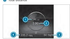
Instrument Display with color display Trip computer (example)
