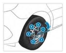
Tighten the wheel bolts or nuts evenly in the sequence indicated (1) to (3).
