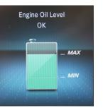
Your vehicle oil level is checked via the On-board computer in the instrument cluster. Park vehicle on level ground. Select in Instrument cluster "service menu > oil level check" Add oil only when indicated. Must be MB specification.
