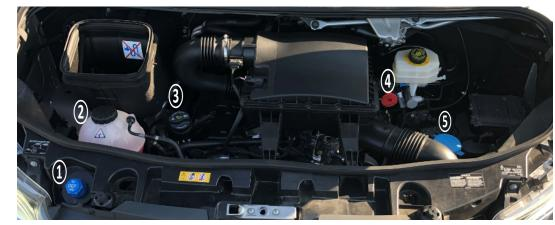
① DEF filler neck cap ② Coolant expansion tank ③ Engine oil filler cap
