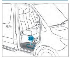
The hydraulic jack is located in side compartment () above the co-driver door step.
