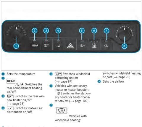
(i) The indicator lamps on the buttons signal that the function in question has been activated.
