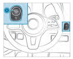
To switch on the power supply: press button () once.
