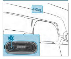
• Switches rear compartment/cargo compartment lamp on or off
