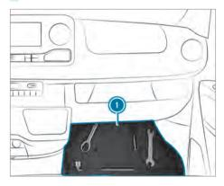
Remove insert ① with the vehicle tool kit.
