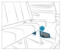
Depending on the vehicle equipment, there will be an air duct or a heater with additional air nozzles in the rear footwell on the left-hand side (). No objects may be placed there. Passengers must maintain a sufficient distance due to the warm air flow and air intake.
