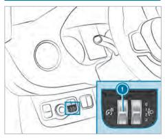
Turn brightness control knob (1) upwards or downwards.
