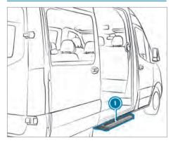
Your vehicle's sliding door may be equipped with an electrical step.
