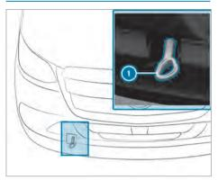
Installing and removing the front towing eye
