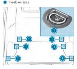
Cargo tie-down points (example: Cargo Van without loading rails)
