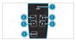
Electronic level control performs a self-check regularly when it is activated and while in use. Indicator lamp () on the remote control lights up for approximately one second when you switch on either the ignition or electronic level control with button ().
