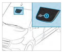
Lane Keeping Assist monitors the area in front of your vehicle with multifunction camera (). It serves to protect you against unintentionally leaving your lane. You may also be warned by a vibrating message from the steering wheel and by the status symbol flashing in the instrument display. The warning is issued when the following conditions are met at the same time:
