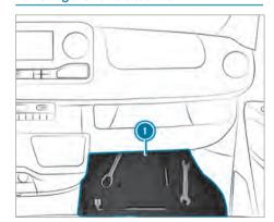
Remove the vehicle tool kit from stowage compartment 1.
