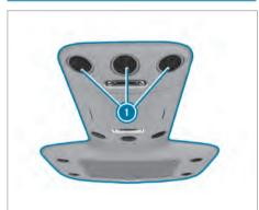
In vehicles with rear-compartment air conditioning, adjustable air vents have been integrated in the roof air duct.
