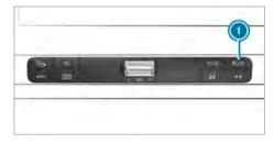
► To switch off: briefly press button ①. The Ⅰ symbol appears in the status line of the multimedia system display.
