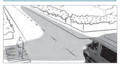
Cornering light improves the illumination of the road over a wide angle in the turning direction, enabling better visibility in tight bends, for example. The function is active under the following conditions:
