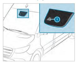
Lane Keeping Assist monitors the area in front of your vehicle with multifunction camera ①. It serves to protect you against unintentionally leaving your lane. You may also be warned by a vibrating message from the steering wheel and by the status symbol flashing in the instrument display.
