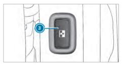
Sliding door button on the door sill (B-pillar) On vehicles with a partition, button (3) is located on the partition next to the doorway at the level of the inside door handle.
