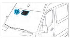
Traffic Sign Assist detects traffic signs with multifunction camera (). It assists you by displaying detected speed limits and overtaking restrictions in the instrument cluster.
