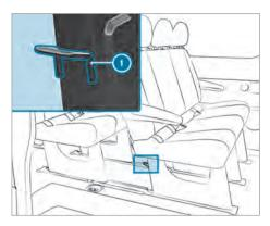
Top Tether anchorages 0 are located on the back of the rear bench seat on the bench seat legs.
