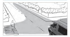
Cornering light improves the illumination of the road over a wide angle in the turning direction, enabling better visibility in tight bends, for example.
