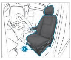
You can rotate the driver's and front-passenger seat 50 ° and 180 °. The seats engage both in and opposite to the direction of travel as well as at 50 ° to the exit.
