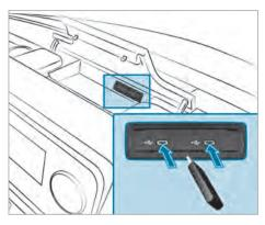
The multimedia connection unit is found in the stowage compartment in the center console and has two type C USB ports.
