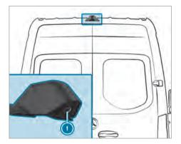
If you have activated the function in the multimedia system, the image from rear view camera 1 appears in the multimedia system when reverse gear is selected. Dynamic guide lines show the path the vehicle will take with the steering wheel in its current position. This helps you to orient yourself and to avoid obstacles when backing up.
