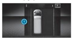
If a lane-correcting brake application from Active Lane Keeping Assist occurs, display ① appears in the multifunction display.
