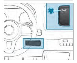
To engage/disengage: press the upper section of switch (a).
