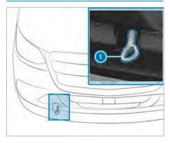
Installing and removing the front towing eye
