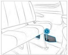
Depending on the vehicle equipment, there will be an air duct or a heater with additional air nozzles in the rear footwell on the left-hand side ①. No objects may be placed there. Passengers must maintain a sufficient distance due to the warm air flow and air intake.
