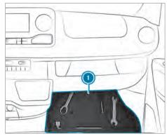
Remove insert 1 with the vehicle tool kit.
