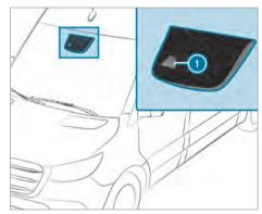
Active Lane Keeping Assist monitors the area in front of your vehicle by means of multifunction camera 1. It serves to protect you against unintentionally leaving your lane. You may also be warned by a vibrating message from the steering wheel and by the status symbol flashing in the instrument display. In addition, you may be guided back into your lane by a lane-correcting brake application. A relevant message appears in the instrument display.
