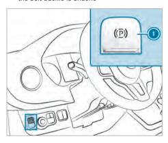
To prevent the electric parking brake from applying automatically, pull switch 1.
