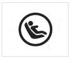
Symbol for installing a LATCH-type (ISOFIX) child restraint system
