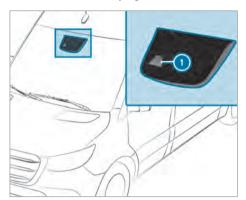
Lane Keeping Assist monitors the area in front of your vehicle with multifunction camera 1. It serves to protect you against unintentionally leaving your lane. You may also be warned by a vibrating message from the steering wheel and by the status symbol flashing in the instrument display.
