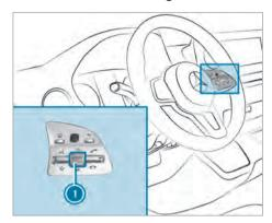
Turn volume control 1. The volume of the current radio or media source is set. The volume of other audio sources can be adjusted separately.
