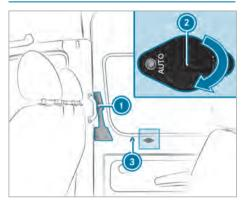
If there has been a malfunction or if the battery has been disconnected, you can use release catch ② to disconnect the sliding door from the electric motor. Then, you can open or close the door manually.
