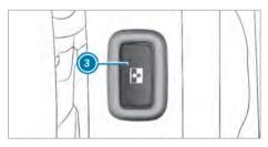
Sliding door button on the door sill (B-pillar) On vehicles with a partition, button (3) is located on the partition next to the doorway at the level of the inside door handle.
