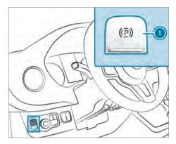
In the event of an emergency, you can brake the vehicle while it is in motion with the electric parking brake.
