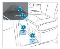
To install: press pushbuttons (1) onto holders (2).
