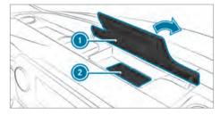
Open the flap of stowage compartment ① above the media display.
