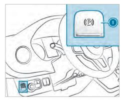
To prevent the electric parking brake from applying automatically, pull switch ①. The electric parking brake is also automatically applied if Active Distance Assist DISTRONIC has brought the vehicle to a standstill.
