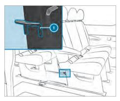
Top Tether anchorages 0 are located on the back of the rear bench seat on the bench seat legs.
