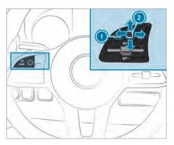
The on-board computer is operated via left-hand Touch Control (2) and the back button on the left (1).
