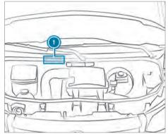
Engraved VIN () is located underneath the hood.
