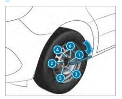
Tighten the wheel bolts or nuts evenly in the sequence indicated (① to ③).
