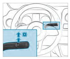
Depress the brake pedal and push the DIRECT SELECT lever upwards past the first point of resistance. Transmission position display R is shown in
