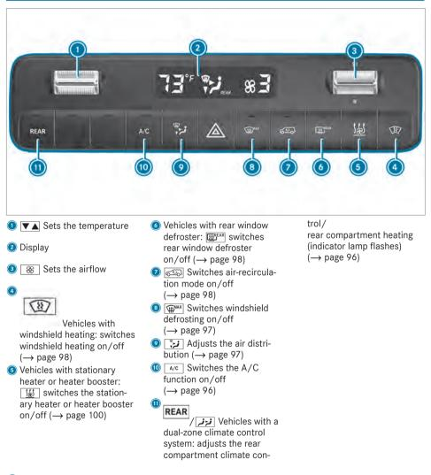
(i) The indicator lamps on the buttons signal that the function in question has been activated.
