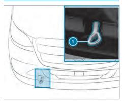
Installing and removing the front towing eye
