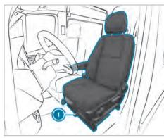
You can rotate the driver's and front-passenger seat 50  $^{\circ}$  and 180  $^{\circ}$ . The seats engage both in and opposite to the direction of travel as well as at 50  $^{\circ}$  to the exit.
