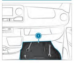
Remove the vehicle tool kit from stowage compartment ①.
