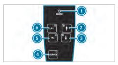
Electronic level control performs a self-check regularly when it is activated and while in use. Indicator lamp ① on the remote control lights up for approximately one second when you switch on either the ignition or electronic level control with button ②.
