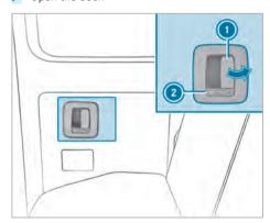
The symbol indicates that the rear door is unlocked.
