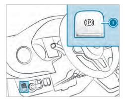
In the event of an emergency, you can brake the vehicle while it is in motion with the electric parking brake.
