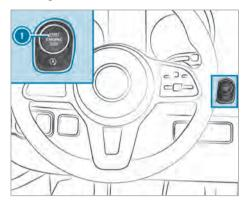
To switch on the power supply: press button
