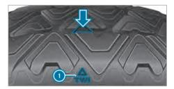
Markings (1) show in which places the bar indicators (arrow) are integrated into the tire tread. They are visible as soon as the tread depth is approximately 1/16 in (1.6 mm).
