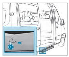
On both sides, insert spring cotters (1) through the housing's holes and into the step as far as they will go.
