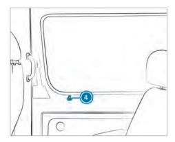
When the sliding door is locked, it can only be opened from the inside by manually unlocking locking pin (4).
