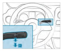
The automatic transmission shifts through the individual gears automatically when it is in transmission position  $\boxed{\textbf{D}}$ . This is determined by the following factors:
