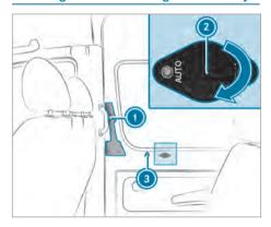
If there has been a malfunction or if the battery has been disconnected, you can use release catch ② to disconnect the sliding door from the electric motor. Then, you can open or close the door manually.
