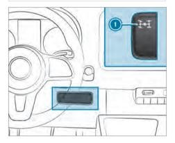
To engage/disengage: press the upper section of switch 1. The indicator lamp in switch (1) flashes while the all-wheel drive is engaged or disengaged. The 📻 and 🔘 warning lamps light up in the instrument display. ESP® and ASR are deactivated for the duration of the shift operation. If the shift operation is successful, the 🚊 and 🔘 warning lamps in the instru-
