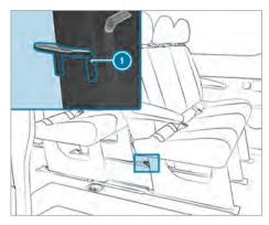
Top Tether anchorages ① are located on the back of the rear bench seat on the bench seat legs.
