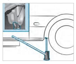
Jack support point, rear axle (example: Cargo Van and Passenger Van up to 4.0 t)
