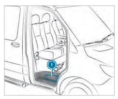
The tire-change tool kit is located in stowage compartment
