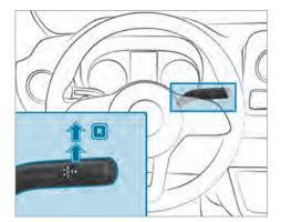
Depress the brake pedal and push the DIRECT SELECT lever upwards past the first point of resistance.
