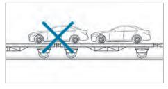
Make sure that the front and rear axles come to rest on the same transportation vehicle.
