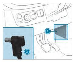
Press plug ② onto the ground pin until you feel it engage and plug ② is in full contact with the ground pin.
