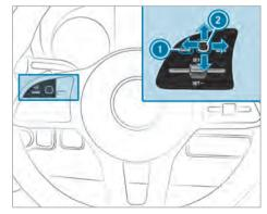
The on-board computer is operated via left-hand Touch Control ② and the back button on the left ①.
