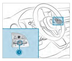
Turn volume control 1. The volume of the current radio or media source is set. The volume of other audio sources can be adjusted separately.
