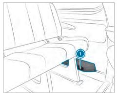
Depending on the vehicle equipment, there will be an air duct or a heater with additional air nozzles in the rear footwell on the left-hand side 1. No objects may be placed there. Passengers must maintain a sufficient distance due to the warm air flow and air intake.
