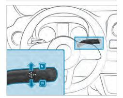
Press the brake pedal and the DIRECT SELECT lever upwards or downwards to the first point of resistance.
