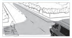
Cornering light improves the illumination of the road over a wide angle in the turning direction, enabling better visibility in tight bends, for example.
