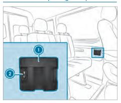
Place the mobile phone in stowage compartment (a) and connect it to USB socket (a) to charge.
