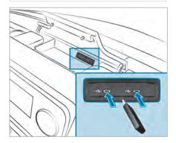
The multimedia connection unit is found in the stowage compartment in the center console and has two type C USB ports.
