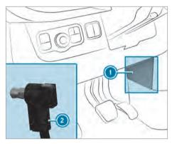
Press plug ② onto the ground pin until you feel it engage and plug ③ is in full contact with the ground pin. All starter battery consumers are reconnec-
