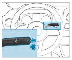
Press button ①. Transmission position display P is shown in the multifunction display.
