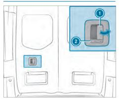
The  $\square$  symbol indicates that the rear-end door is unlocked.
