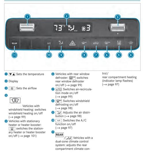
(i) The indicator lamps on the buttons signal that the function in question has been activated.
