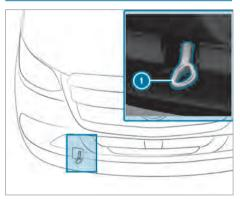
Installing and removing the front towing eye
