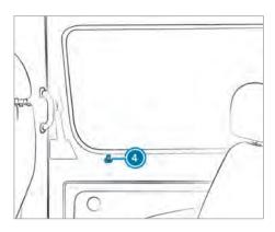
When the sliding door is locked, it can only be opened from the inside by manually unlocking locking pin ().
