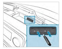
The multimedia connection unit is found in the stowage compartment in the center console and has two type C USB ports.
