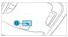
When the ATA system is armed, indicator lamp ① flashes in the overhead control panel.
