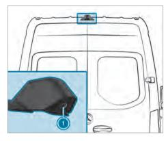
If you have activated the function in the multimedia system, the image from rear view camera () appears in the multimedia system when reverse gear is selected. Dynamic guide lines show the path the vehicle will take with the steering wheel in its current position. This helps you to orient yourself and to avoid obstacles when backing up.
