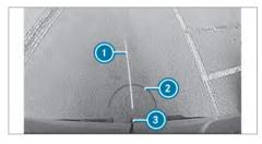
View of trailer (if trailer hitch is installed) Yellow guide line, locating aid
