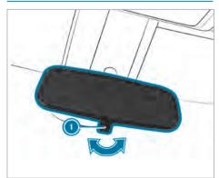
To dim the inside rearview mirror: move anti-glare lever () in the direction of the arrow.
