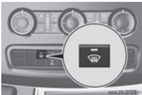
Windshield heater switch
