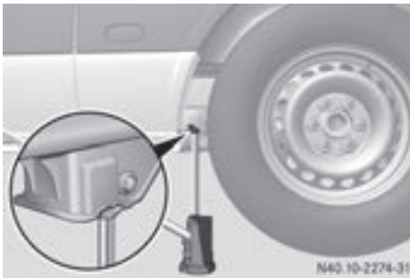
Jacking point, rear axle (example: vehicle type 3500)
