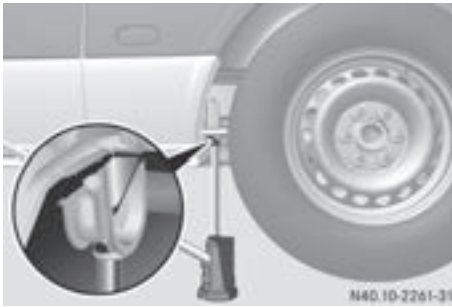
Jacking point, rear axle (example: vehicle type 2500)
