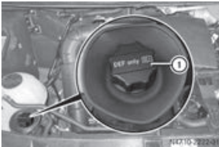
Example: DEF filler cap in the engine compartment
