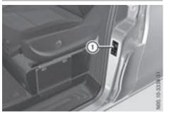
Vehicle identification plate on the driver's side B-pillar
