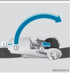
Tensioning lever fastened in detent position
