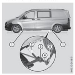
Jacking points ① (rubber stoppers) are located just behind the front wheel arches and just in front of the rear wheel arches.
