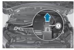
► Push contact protection cover ① of the jumpstarting connection point backwards against the spring force as far as it will go. The jump-starting connection point is visible.
