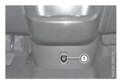
When the key is turned to position 1 in the ignition lock, the sockets can be used for accesso-
