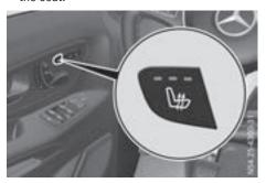
The three red indicator lamps in the button show the activated heating level 1 to 3.
