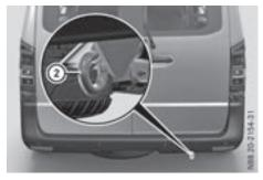
The rear towing eye is located under the bumper.
