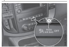
PASSENGER AIR BAG OFF indicator lamp ① shows you whether the front-passenger front air bag is deactivated.
