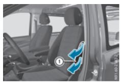
Side impact air bags (1) deploy next to the outer bolster of the seat backrest.
