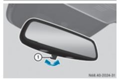
► Anti-glare mode: push anti-glare lever ① forwards or back.
