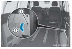
Stowage compartment in the rear on the right-hand side of the vehicle
