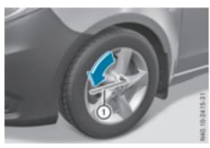
▶ Using lug wrench ①, loosen the wheel bolts on the wheel to be changed counter-clockwise by about one full turn. Do not remove the wheel bolts.
