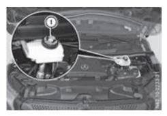
Check the brake fluid level regularly, e.g. weekly or when refueling.
