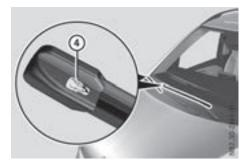
► Remove protective film ④ from the service indicator on the tip of the wiper blades.
