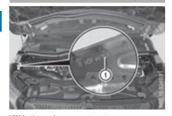
VIN in the engine compartment
