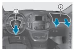
Driver's air bag (1) deploys in front of the steering wheel. Front-passenger front air bag (2) deploys in front of and above the glove box and the center console.
