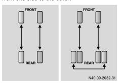
Diagram showing tire rotation for single and dual tires
