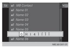
► To find a contact: enter the initial letter of the desired contact by using the 2/msc to 9/msz number keys.
