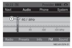
► Press and hold a number key from 2 to until the display shows the number in front of the station frequency or station name (1).
