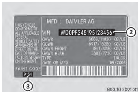
Example: vehicle identification plate (US vehicles)
