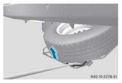
1 You can raise the spare wheel bracket or lower it to the ground using the jack pump lever as shown.
