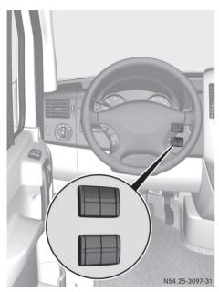
Switch unit between the steering wheel and ignition lock
