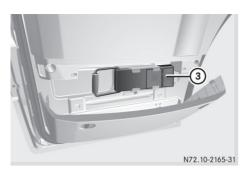
The warning lamp is behind the cover in the storage compartment of the driver's door.
