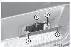
Tire sealant in the stowage compartment in the right-hand door sill
