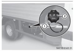
DEF tank on the right-hand side of the vehicle (example: Cab Chassis)
