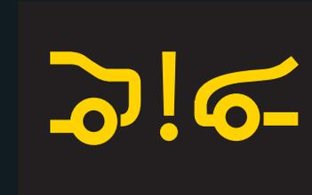
COLLISION PREVENTION ASSIST<sup>®12</sup> is a radar-based proximity warning system that issues visual and audible warnings when vehicles traveling ahead come within a potentially dangerous distance. In emergency situations, boosted braking pressure levels assist automatically to help prevent rear-end collisions.
